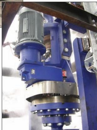
Figs. 3. and 4. Electrical driven decoking hoist (left hand and right hand version) and electrical driven drill stem drive.
