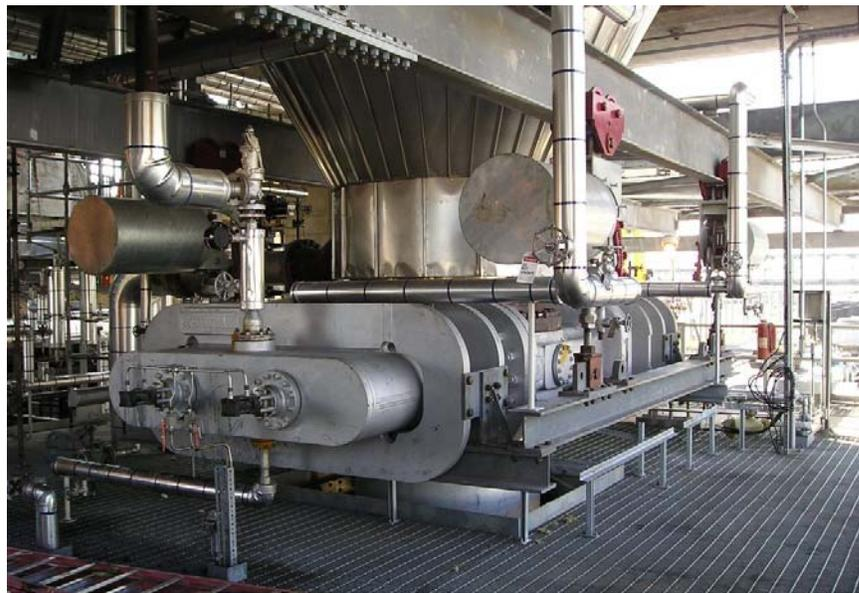
Fig. 5 – Frontier's Bottom Unheading Valve, Deck and Monorail System
