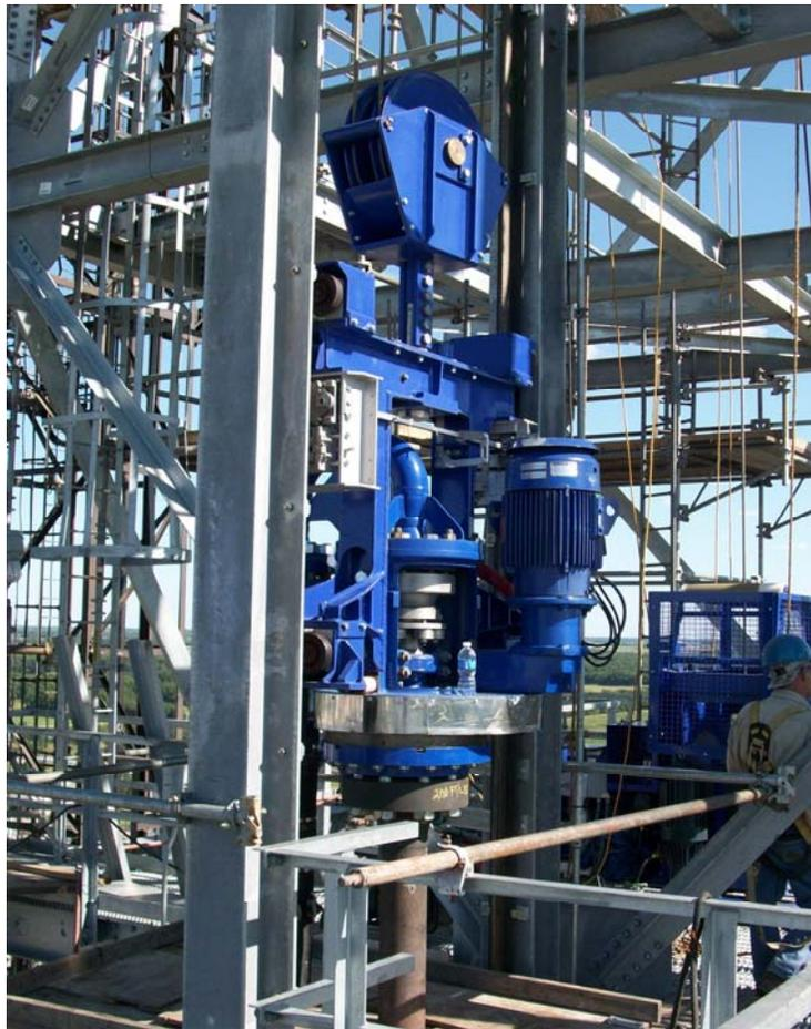
Fig. 10 – Decoking System Drill Stem Drive
